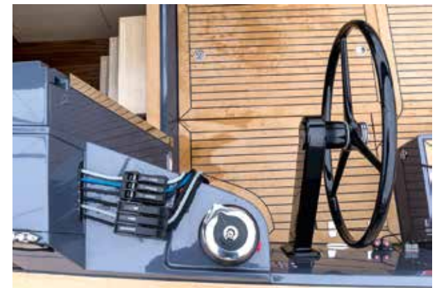
Above: under-deck sheets exit directly in front of clutches and winch Left: adjustable helm foot brace hinges up from the cockpit sole
