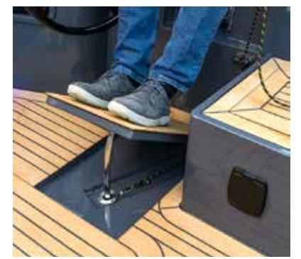
Above: under-deck sheets exit directly in front of clutches and winch Left: adjustable helm foot brace hinges up from the cockpit sole
