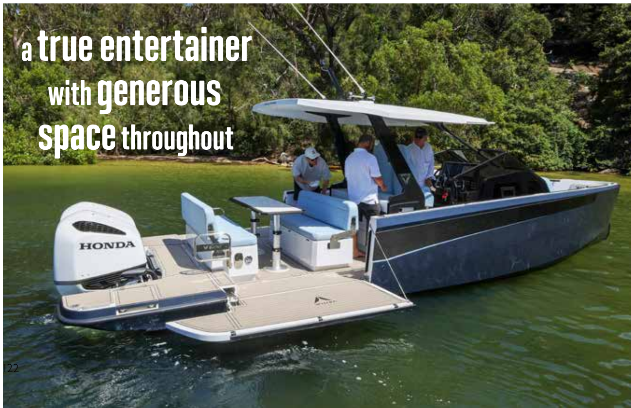
Below: Foldable balconies significantly extend the 2.9m hull beam when at rest.
