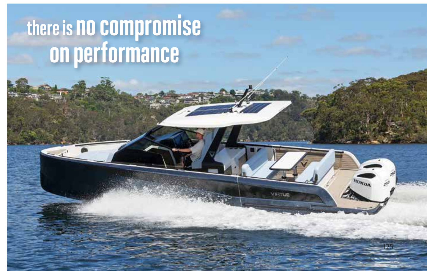
Below: Swedish Petestep hull technology enhances efficiency and reduces power demands. With twin Honda 25s the V10 achieves nearly 50 knots.
