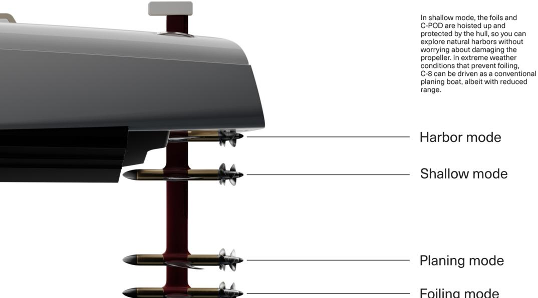
In harbor mode, the foils fully retract above the water surface and are therefore protected from fouling and corrosion. This mode also makes C-8 trailerable and compatible with boat lifts.
